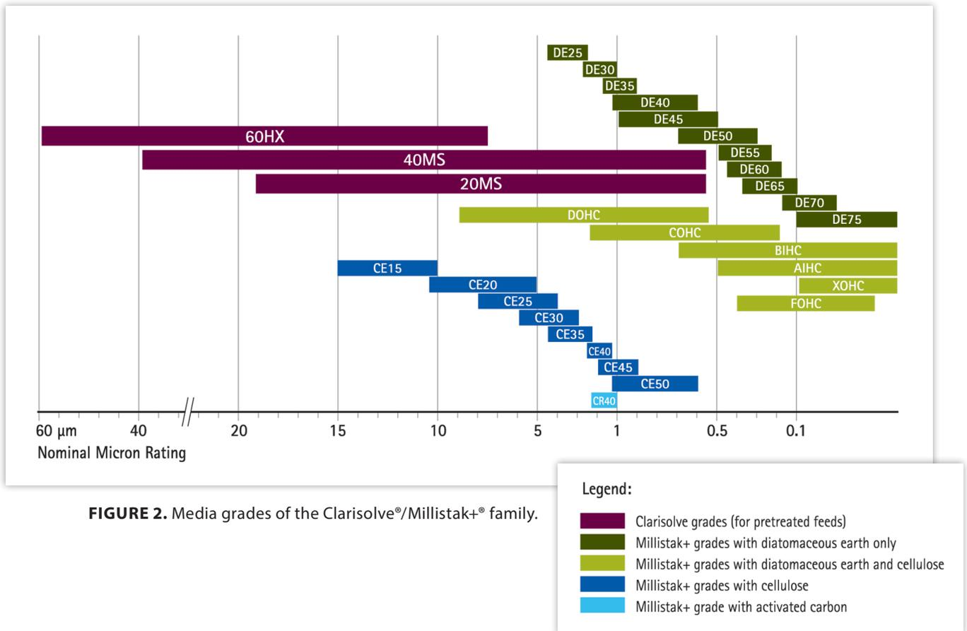
**FIGURE 2.** Media grades of the Clarisolve®/Millistak+® family.
