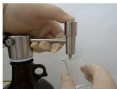
Place a receptacle under the outlet and withdraw the solvent by pushing the valve downwards. The valve closes automatically when stop pushing it.
