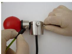
Attach the antistatic cable to a safe ground connection and connect it to the withdrawal system.
