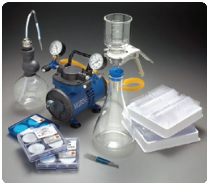
Figure 23. Laboratory Filter Apparatus assembled using the Fluid Contamination Kit (Cat Nos. XX7104711K and XX7104712).
