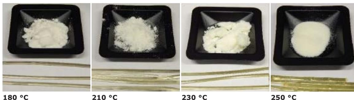
**Figure 7:** Visual comparison of Parteck® MXP extrudate at various temperatures
