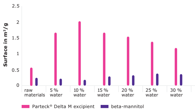
Fig. 2: BET surface – granules of delta- vs. beta-mannitol produced by wet granulation.
