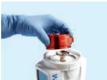
Place rotor on instrument
