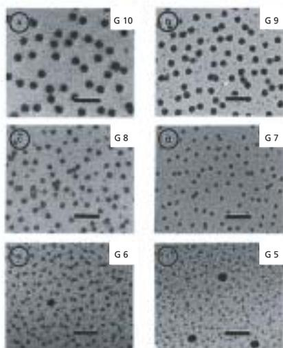
**Figure 9.** Transmission Electron Micrographs (TEMs) of Gen 5–10 PAMAM Dendrimers. Sample ① Contains Three Molecules of Gen 10 Dendrimer for Comparison. Bar Length = 50 nm. (Reproduced from Reference 80 with Permission from ACS.)
