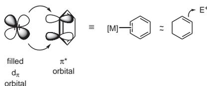
Figure 1. Fundamental Metal–Ligand Interaction and Activation. (Ref. 12)
