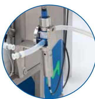
Pre-column instrumentation for conductivity and pH measurement
