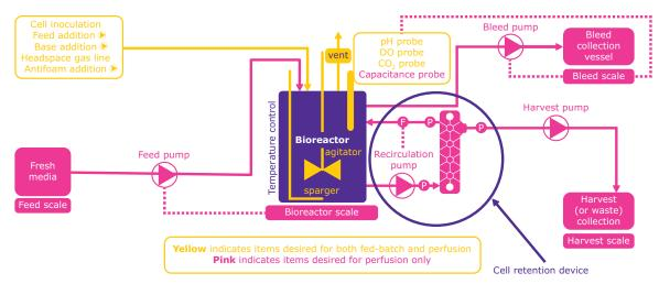
Figure 6. A cell retention device is critical to derive the greatest benefit from perfusion approaches.
