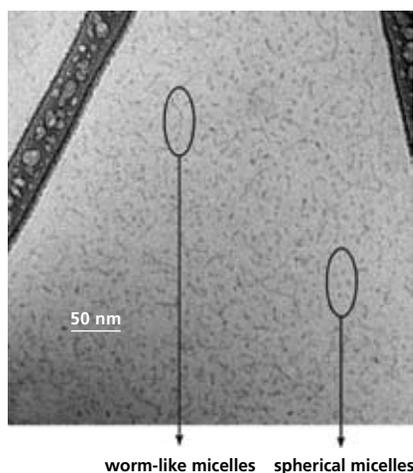
**Figure 5.** Cryo-TEM Image of PTS-H<sub>2</sub>O. (Photo © B. H. Lipshutz.) (Ref. 25,26)
