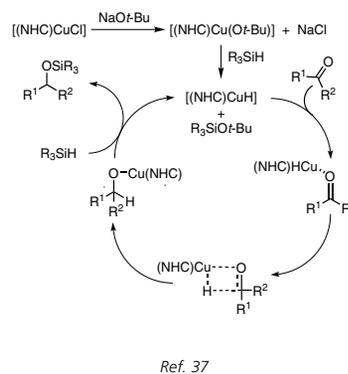
**Scheme 4.** Proposed Mechanism for the [(NHC)CuCl]-Catalyzed Hydrosilylation of Ketones.
