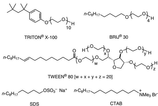
**Figure 2.** Commonly Used Nonionic and Ionic Surfactants.
