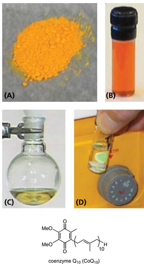
**Figure 4.** (A) Pure, Water-Insoluble Coenzyme Q<sub>10</sub>. (B) Solution of 50 mg/mL CoQ<sub>10</sub> in PTS-H<sub>2</sub>O. (C) Neat PTS. (D) Solution of TAXOL® in PTS-H<sub>2</sub>O (10 mg/mL). (Photos © B. H. Lipshutz.)
