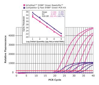
Target gene was amplified from log-fold dilutions of total HeLa cell cDNA (100 ng to 10 pg) using KiCqStart® SYBR® Green qPCR ReadyMix $^{\text{TM}}$  or Competitor Q according to each manufacturer's protocol. Plots represent averages of quadruplicate reactions.
