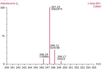
The significantly improved mass spec performance of the d<sub>4</sub> standard is clearly seen when the molecular ions of aldosterone, aldosterone-d<sub>4</sub>, and aldosterone-d<sub>7</sub> are superimposed (see **Figure 8**). Two ions are shown for the d<sub>7</sub> standard since both the d<sub>7</sub> and d<sub>8</sub> ion could be chosen. Clearly the d<sub>4</sub> standard is the internal standard of choice.
