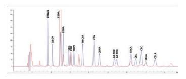
Figure 4. Overlay of Hemp Sample and Peak Identification Mix, Isocratic Method on Ascentis Express C8 2.7  $\mu m$  Column
