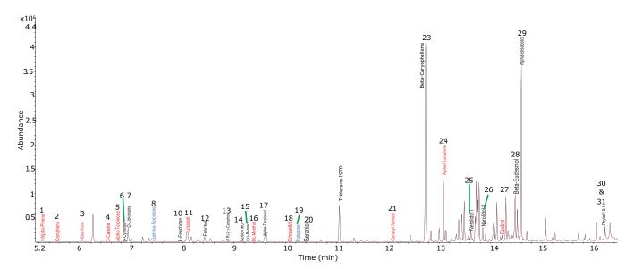
Figure 5. Chromatogram of GC-MS Analysis of Hemp Extract.
