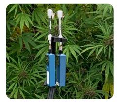
Figure 2. Outdoor measurement of terpenes from hemp growing operations using a glass and a stainless steel Carbotrap® T420 TD tube and a Spectrex PAS-500 Personal Air Sampling pump.
