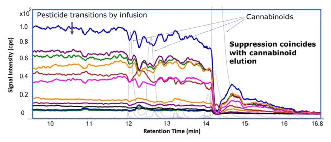
**Figure 4**. A portion of the Chromatographic Run in a Tee-Infusion Experiment - The colored traces indicate the signal intensity of several pesticides being infused over the course of a run. The cannabinoid peaks (grey) were collected as a separate chromatographic run and have been overlaid with the infusion data for illustration. The suppression occurring after 15 minutes is due to unidentified matrix components eluting from the column.
