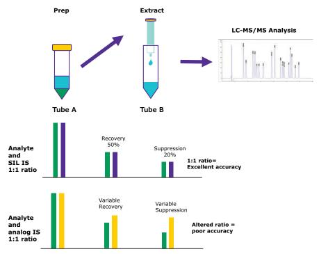
Figure 6. A Depiction of the Advantages Obtained by Use of SIL IS Over Analog IS in LC-MS/MS Analysis.
