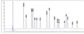
Figure 2. Separation of Cannabinoids in the Peak Identification Mix Using a Gradient on a 2.7  $\mu m$  Ascentis® Express C18 Column
