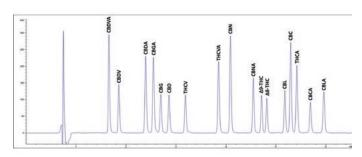
Figure 1. Separation of Cannabinoids in the Peak Identification Mix Using a Gradient on a 2  $\mu m$  Ascentis® Express C18 Column
