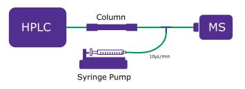
Figure 2. Illustration of Tee-Infusion Experimental Set-Up
