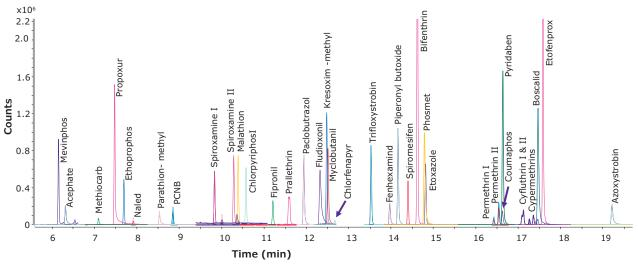
Figure 5. Standard Injection of California Pesticides Prepared in Hemp and Analyzed by GC-MS/MS
