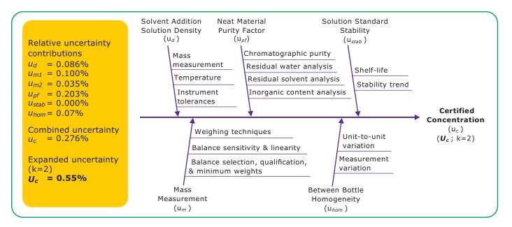
Figure 2. Example fishbone diagram of measurement uncertainty contributions for a gravimetrically prepared CRM.
