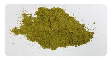
Figure 2. Hemp Buds "Finola" after Grinding in a Cryo Ball Mill. Resulting Particle Size <100  $\mu m.$
