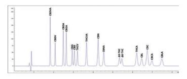
Figure 3. Separation of Cannabinoids in the Peak Identification Mix Using an Isocratic Method on a 2.7  $\mu m$  Ascentis® Express C8 Column.
