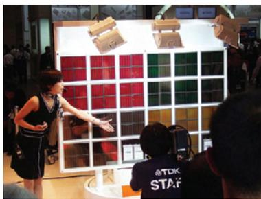
**Figure 3.** Tuning of colors of dye-sensitized solar cell. Printed with permission from Schott AG.
