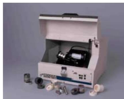
**Figure 1.** A planetary mill Pulverisette 5 / 4, Fritsch (top) and a shaker mill Spex 8000M (bottom). Images provided by manufacturers.
