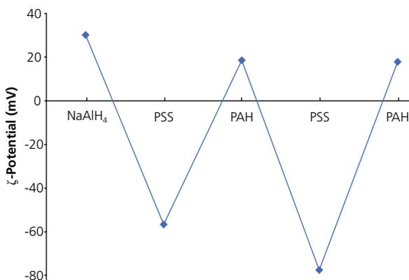
**Figure 3.** Zeta potential measurement from sodium aluminum hydride having PSS and PAH overlay films (two polymeric bilayers).
