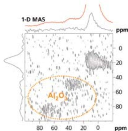
**Figure 3.** Two-Dimensional (2D) MQMAS <sup>27</sup>Al spectrum of  $\alpha$ -AlH<sub>3</sub> ( $\omega_r=35$  kHz) shows two weaker peaks at ~40 ppm and ~65 ppm from 5-fold and 6-fold Al-O sites in addition to the peak at 6 ppm from the hydride.
