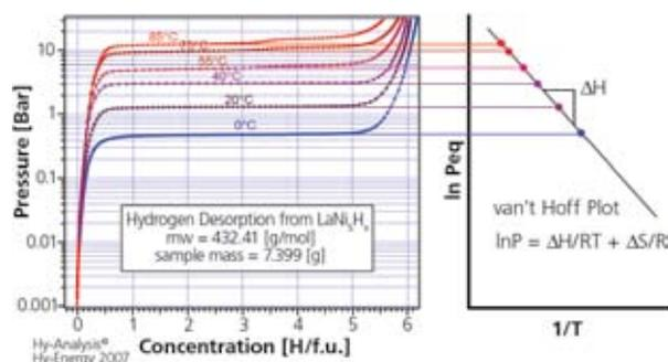
**Figure 3.** PCT curves and van't Hoff plot for  $\text{LaNi}_5$ .<sup>3</sup>
