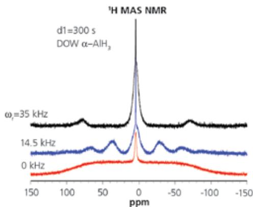
Figure 1. Static and  $^1\text{H}$  MAS NMR spectra of  $\alpha$  phase aluminum hydride ( $\alpha\text{-AlH}_3$ ) obtained at the resonance frequency of 500.23 MHz. (bottom) static (0 kHz)  $d_1=300$  s, (middle) MAS (14.5 kHz),  $d_1=300$  s, (top) MAS (35 kHz),  $d_1=300$  s, where  $d_1$  is the repetition delay time during signal averaging.
