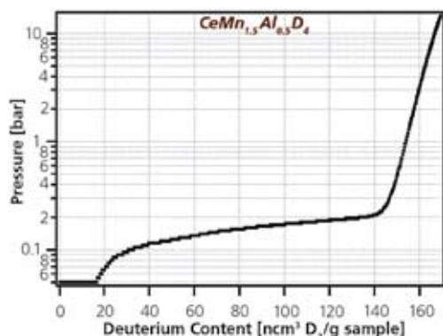
Figure 4b. Deuterium capacity correlated with neutron diffraction patterns.
