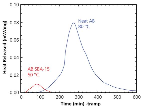
Figure 5. Isothermal DSC comparisons showing lower reaction enthalpy for H<sub>2</sub> loss from AB on mesoporous silica SBA-15.
