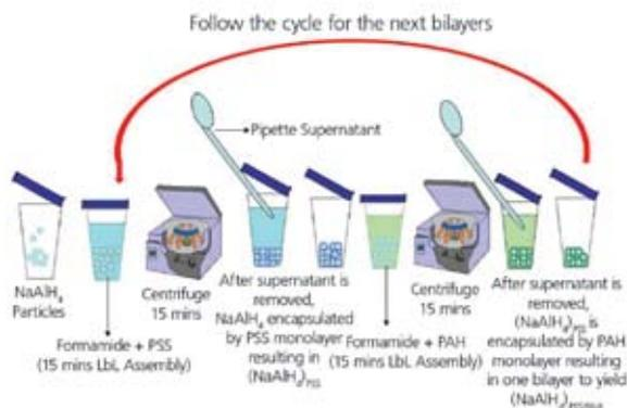
**Figure 2.** The process of coating “smart” nanofilms onto sodium aluminum hydride.
