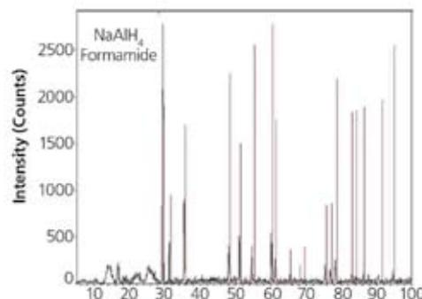
**Figure 5.** X-ray diffraction of NaAlH<sub>4</sub> after 24 hour soak in formamide—the working solvent.
