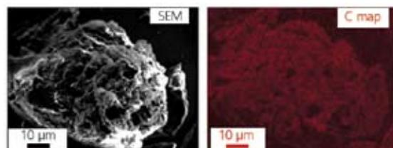
**Figure 4.** SEM and X-ray mapping of carbon (from nanofilms) on sodium aluminum hydride.
