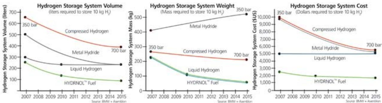
Figure 4. Comparison of On-Board Hydrogen Storage Systems
