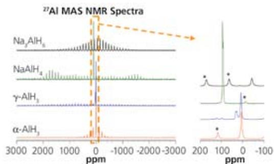
Figure 2.  $^{27}\text{Al}$  MAS NMR spectra of  $\alpha$  and  $\gamma$  phases of  $\text{AlH}_3$ ,  $\text{NaAlH}_4$  and  $\text{Na}_3\text{AlH}_6$  obtained at the resonance frequency 130.35 MHz with strong  $^1\text{H}$  decoupling.
