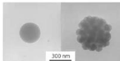
**Figure 7.** 250 nm diameter bare latex particle (left) and covered with 40-nm silica particle shell (PAH/PSS/PAH/silica) (right).
