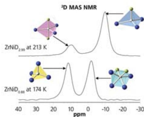
**Figure 4.** Rigid-lattice <sup>2</sup>D MAS NMR spectra ( $\nu_r=76.79$  MHz) for the  $\gamma$ -ZrNiD<sub>2.99</sub> (upper) and the  $\beta$ -ZrNiD<sub>0.88</sub> (lower). Spinning sidebands are not shown in both spectra. The fits to these spectra yield two distinct resonances for each phase that correspond to the indicated D sites as described in Ref. 23.
