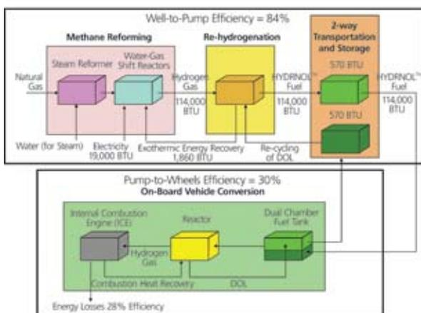
Figure 3. Well-to-Wheels Estimate for Asemblon's HYDRNOL™ Fuel.
