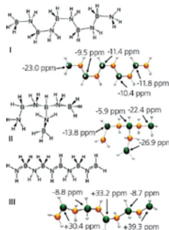
**Figure 3.** The possible structures arising from dehydropolymerization of AB using DFT/GIAO calculated values of  $^{11}\text{B}$  NMR. Reprinted with permission from Ref. 18 ©2006 American Chemical Society.
