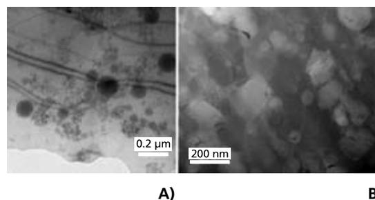
**Figure 2.** TEM of Aluminum Alloy- $\text{Al}_2\text{O}_3$  nanocomposites produced by liquid and solid based methods. A) Stir cast A206- 2 vol %  $\text{Al}_2\text{O}_3$  (47 nm) nanocomposite produced by the authors at UW–Milwaukee.<sup>7</sup> B) Powder metallurgy based Aluminum alloy-15 vol%  $\text{Al}_2\text{O}_3$ .<sup>8</sup>
