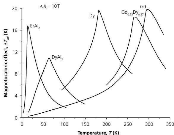
**Figure 4.** The magnetocaloric effect in  $\text{ErAl}_2$ ,<sup>8</sup>  $\text{DyAl}_2$ ,<sup>8</sup>  $\text{Dy}$ ,<sup>9</sup>  $\text{Gd}_{0.73}\text{Dy}_{0.27}$ ,<sup>10</sup> and  $\text{Gd}$ <sup>7</sup> calculated from heat capacities measured in a zero and 10 T magnetic field.
