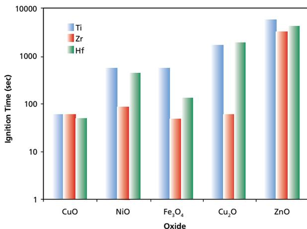
**Figure 4.** Ignition times of Mechanically Induced Self-propagating Reactions between Cu, Ni, Fe and Zn oxides, and Ti, Zr, and Hf metals.
