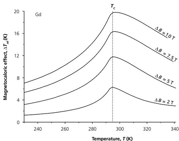
**Figure 2.** The magnetocaloric effect (adiabatic temperature change,  $\Delta T_{ad}$ ) for Gd calculated from heat capacity data.
