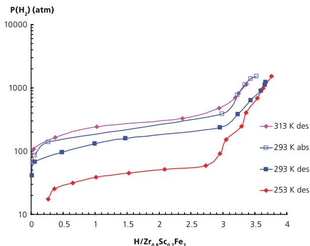
Figure 6. Desorption isotherms for  $\text{Zr}_{0.5}\text{Sc}_{0.5}\text{Fe}_2\text{-H}_2$  system.
