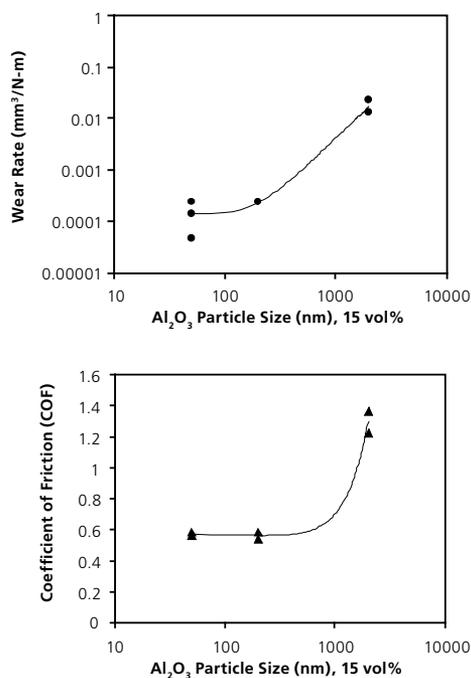
**Figure 3.** Effect of particle size on wear rate and coefficient of friction of Al-15vol% Al<sub>2</sub>O<sub>3</sub> metal matrix composites. Both the wear rate and coefficient of friction are dramatically reduced when the particle size is reduced below 1  $\mu\text{m}$ .<sup>8</sup>
