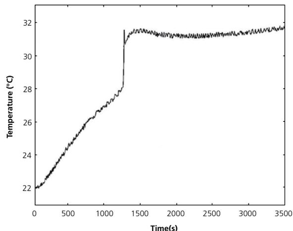
**Figure 2.** Temperature of the outside surface of the vial during ball milling of a 5 Ni + 2 P mixture in a SPEX 8000 Mixer Mill. Ignition is indicated by the rapid temperature rise at 1220 sec. The gradual temperature increase before ignition is caused by dissipated mechanical energy.
