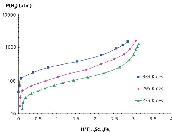
Figure 7. Desorption isotherms for  $\text{Ti}_{0.5}\text{Sc}_{0.5}\text{Fe}_2\text{-H}_2$  system
