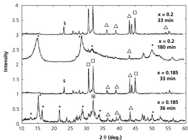
**Figure 3.** X-ray diffractograms of two  $x(\text{Zn+S}) + (1-x)(\text{Sn+2S})$  mixtures. The main lines of Sn ( $\square$ ), Zn ( $\Delta$ ), S, SnS ( $\times$ ),  $\text{SnS}_2$  ( $*$ ) and  $\text{Sn}_2\text{S}_3$  ( $+$ ) are indicated.
