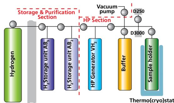
**Figure 1.** Schematic of a high-pressure (HP) system.
