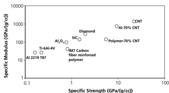
**Figure 1.** Comparison of potential materials and reinforcements for aerospace applications. (Data for Al-70% CNT is theoretical)
