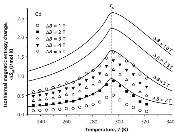
**Figure 1.** A comparison of the magnetocaloric effect (isothermal magnetic entropy change,  $\Delta S_m$ ) for Gd calculated from magnetization (symbols) and heat capacity data (solid lines).
