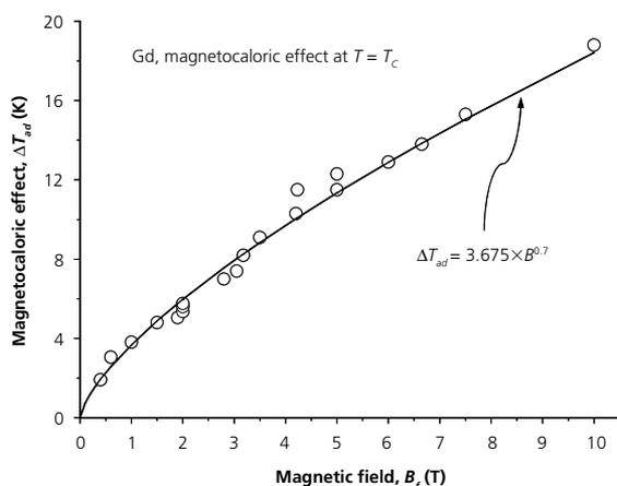
**Figure 3.** The magnetocaloric effect for Gd at its Curie temperature, shown as a function of the final magnetic field,  $B_f$ , for  $B_i = 0$ . The symbols represent values either measured directly or calculated from heat capacity data by different authors.<sup>7</sup> The line is the least squares fit assuming power-law dependence of the MCE on the magnetic field.
