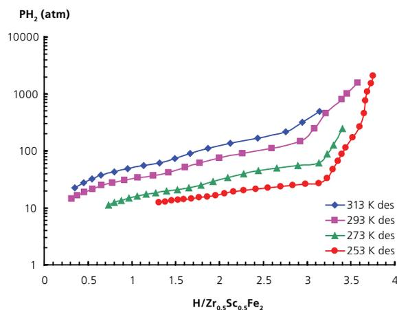
**Figure 5.** Absorption-desorption isotherms for Zr<sub>0.5</sub>Sc<sub>0.5</sub>Fe<sub>2</sub>-H<sub>2</sub> system.
