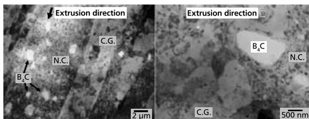
**Figure 4.** TEM micrographs showing alternate stacking of course grain size Al and nanostructured Al regions. The  $B_4C$  particles are uniformly distributed within the nanostructured aluminum exclusively.<sup>16</sup>
