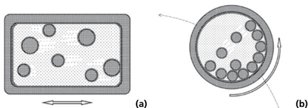
**Figure 1.** Cross section views of the milling vial of a shaker mill (a) and a planetary mill (b).
