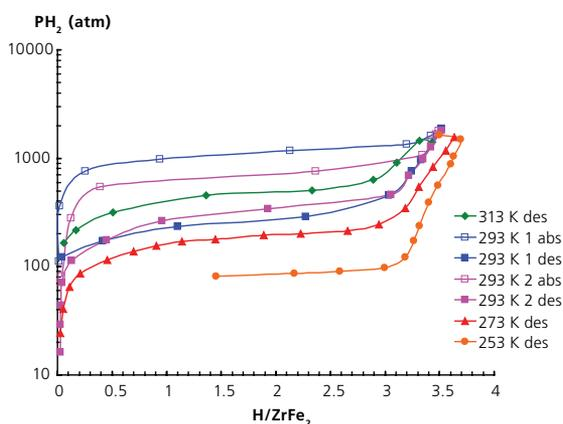
**Figure 4.** Absorption-desorption isotherms for ZrFe<sub>2</sub>-H<sub>2</sub> system.
