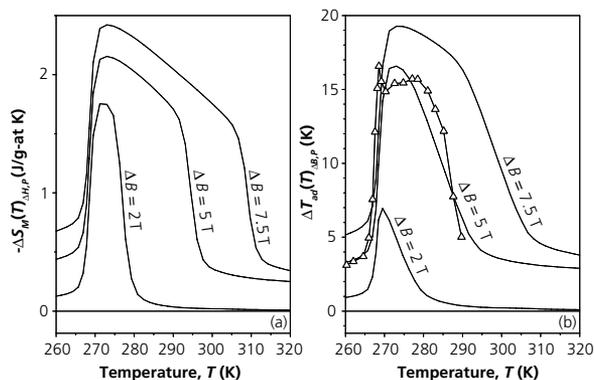
**Figure 5.** The giant magnetocaloric effects in  $Gd_5Si_2Ge_2$  as represented by (a) extensive ( $\Delta S_M$ ) and (b) intensive ( $\Delta T_{ad}$ ) measures, shown as functions of temperature for three different magnetic field changes: from 0 to 2T, from 0 to 5T, and from 0 to 7.5T calculated from heat capacity data. The open triangles in (b) represent the GMCE measured directly for a magnetic field change from 0 to 5T.
