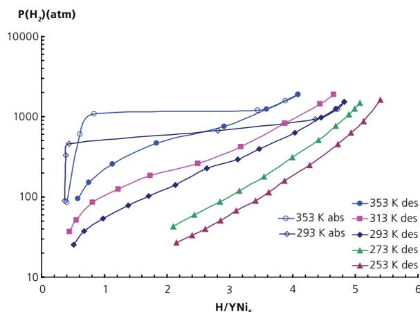
**Figure 2.** Absorption-desorption isotherms for YNi<sub>5</sub>-H<sub>2</sub> system.
