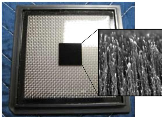
CNT array (black square) in the semiconductor grade package. Inset shows SEM image of the vertically aligned MWCNTs.
