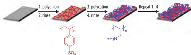
**Figure 1.** Schematic diagram of layer-by-layer adsorption of polyelectrolyte multilayers. The figure also shows the structures of two common polyelectrolytes, poly(styrene sulfonate) and protonated poly(allylamine).
