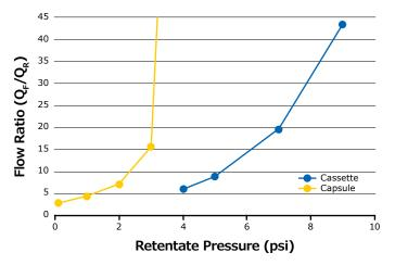
Figure 3. Example of optimal pressure curves for 1 g/L feed at 1 L/min/m<sup>2</sup>.
