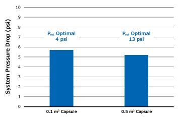
Figure 8. Pressure drop across feed channel for 0.1 and 0.5  $\mbox{m}^{2}$  capsules at 0.84 LMM.
