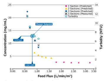
Figure 7. Results of  $0.1\ \text{m}^2$  capsule, 3-section series SPTFF scale-down study.
