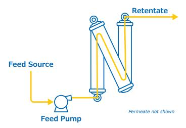
Figure 1. Three capsules in series setup.
