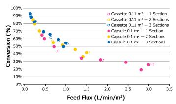
Figure 5. Feed flux excursion for 25 g/L BgG feed solution.
