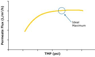
**Figure 2.** Typical batch TMP excursion showing example of ideal operating point for SPTFF.
