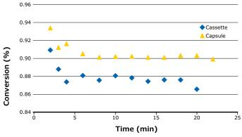
Figure 6. Process stability for SPTFF of 25 g/L BgG run at 0.14 LMM.
