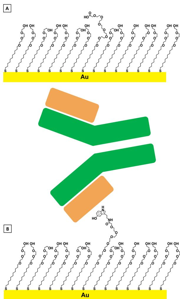
**Figure 11.** (A) The Solution Insertion of Precursor Tether Molecules [Carboxylic Acid Terminated, Oligo(Ethylene Glycol) Functionalized *n*-Alkanethiols] into a Preformed Oligo(Ethylene Glycol) Functionalized *n*-Alkanethiolate SAM. (B) The Capture of a Serotonin Antibody by the 5-HTP Functionalized Tether Molecule.
