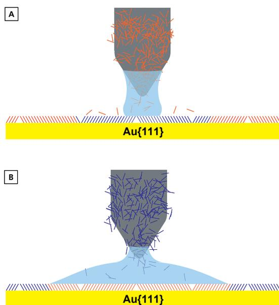
**Figure 9.** Schematic of the Double-Ink, Dip-Pen Nanolithography Experiments. **(A)** The Water Meniscus Was Compact When 16-Mercaptohexadecanoic Acid (MHDA) Molecules (Red) Were Patterned atop a 1-Octadecanethiolate SAM (Blue), Which Resulted in a Lower Transport Rate of the MHDA Molecules. **(B)** The Water Meniscus Was Spread Out When 1-Octadecanethiol Molecules (Blue) Were Patterned atop an MHDA SAM (Red), Which Resulted in a Higher Transport Rate of the 1-Octadecanethiol Molecules.
