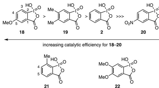
Figure 2. Catalytic Efficiencies of Arene-Substituted IBXs. (Ref. 27)
