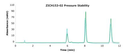
The very good pressure stability is proven with a pressure-shock test showing excellent stability.
