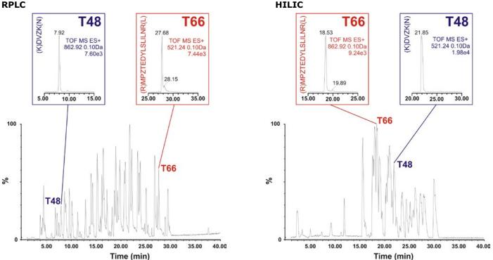
Base peak intensity chromatograms (BPI's) show peptide maps of a BSA tryptic digest using RPLC (left) and ZIC®-HILIC (right) gradients. Inserts show the ion chromatograms of two peptide fragments T48 and T66, (K)DVZK(N) and (R)MPZTEDYLSLILNR(L) respectively. T48 is a smaller peptide fragment with a molecular weight of 520.23 whereas T66 has a molecular weight of 1723.23 (but detected as M+2R ion).
