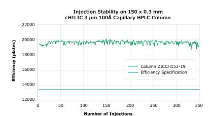
The improved packing results in an extremely good stability of the NEW SeQuant<sup>®</sup> ZIC<sup>®</sup>-HILIC and ZIC<sup>®</sup>-cHILIC capillary columns.
