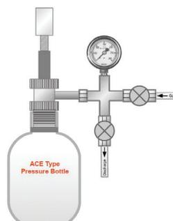
**C** QianCap with gas purging set. When used with Aldrich® lecture-bottle stations, QianCap can be operated easily, safely, and accurately for reaction reproduction with a wide range of gases, including H<sub>2</sub>, D<sub>2</sub>, O<sub>2</sub>, CO<sub>2</sub>, NH<sub>3</sub>, N<sub>2</sub>, Ar, CO, etc.
