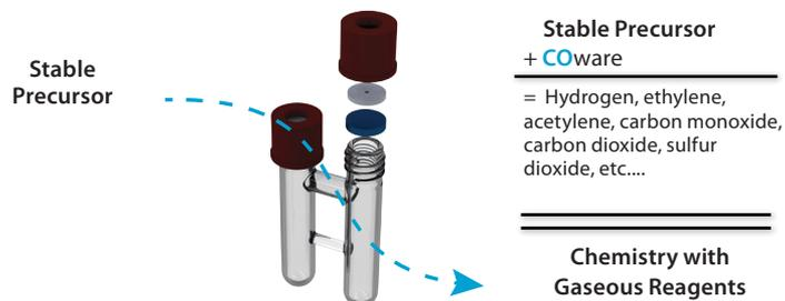
The H-Cap system design makes COware useful for hydrogenation reactions using either generated hydrogen or deuterium gas. Hydrogen or deuterium gas will diffuse through the standard PTFE/silicone seals used for COware, leading to failure of the desired reaction.
