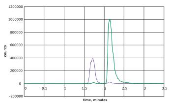
Figure 5. Glyphosate (red trace) and AMPA (blue trace) spiked into oatmeal at 800  $\ensuremath{\mathsf{ppb}}$
