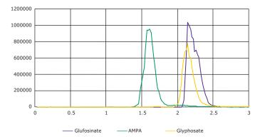
**Figure 3**. LC/MS Analysis of Glyphosate, AMPA, and Glufosinate using Supel<sup>™</sup> Carbon HPLC column. Quantitative transitions are shown for each analyte. Conditions are described in the experimental section. 100 ng/mL calibration standard is shown.
