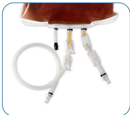
Connection of bag with: inlet tubing, outlet tubing, and injection port (from left to right)
