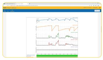
Obtain comprehensive meta data form the Steritest<sup>®</sup> Symbio pump, for example pump speed, pressure or a detailed pump activity profile. This profile can prove that no overpressure has occurred and the Steritest<sup>®</sup> cannisters were not incubated under pressure that could harm microorganisms and thus lead to false negative results.
