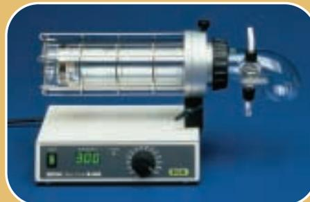
Suitable for drying 100 to 250mL sample volumes, under inert gas or vacuum if required. Drying tube assembly consists of tube which enters oven and end cap fitted with stopcock with vacuum and atmosphere/inert gas connections. Sample is placed in drying tube, which attaches to end cap with vacuum-tight flange. End cap is designed to hold desiccant to absorb water driven off by heat. Oven may also be used for sublimation using optional sublimation insert.
