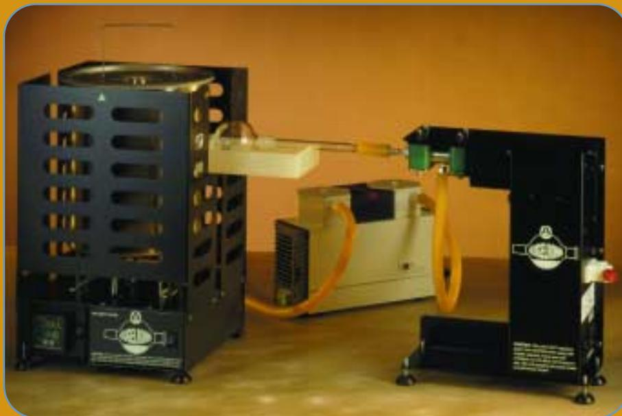
Kugelrohr apparatus shown with KNF Laboport vacuum pump.
