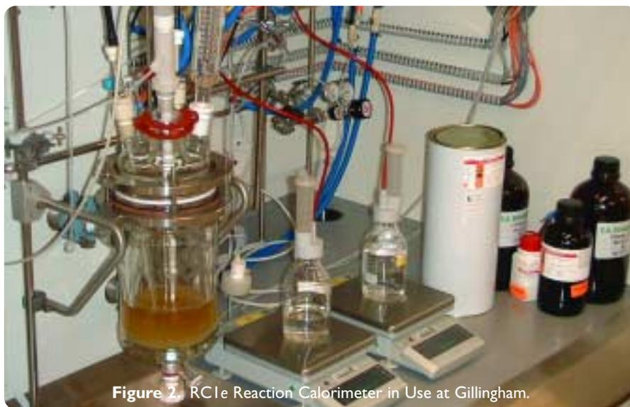
Figure 2. RC1e Reaction Calorimeter in Use at Gillingham.
