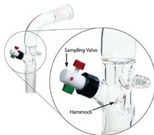
**Figure 1.** Distillate sampling adapter
