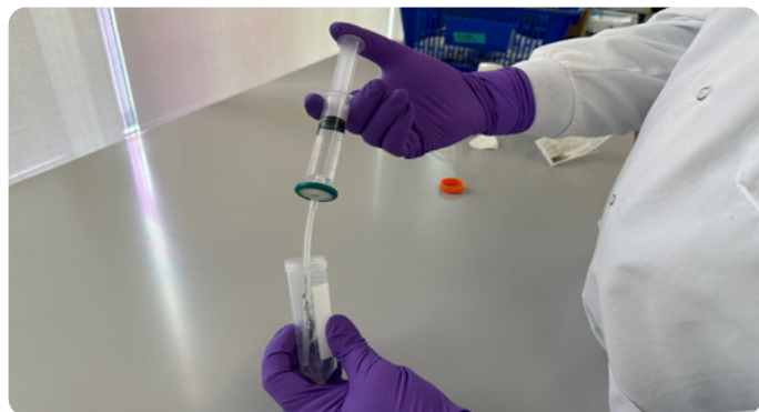
Figure 2. Gentler, pressure-driven microfiltration (top); Syringe virus control microfiltration check (bottom).
