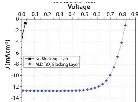
**Figure 5.** Photocurrent density–voltage curve for the mesoscopic perovskite solar cell with (and without) the  $TiO_2$  blocking layer.
