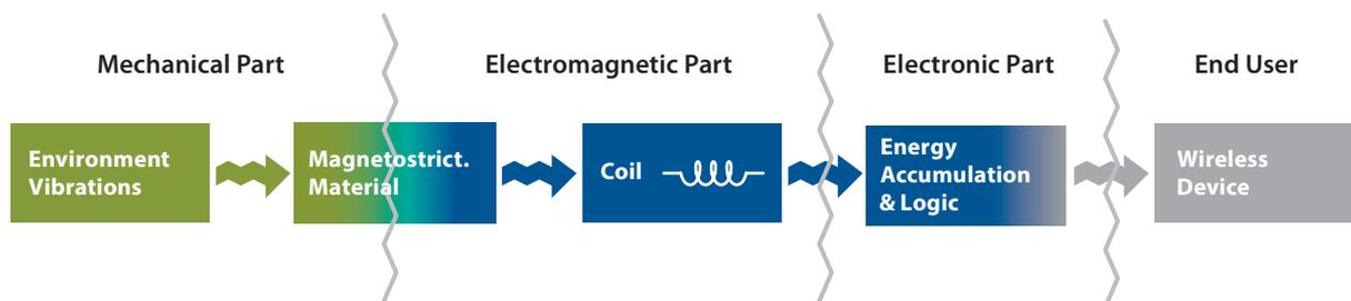
Figure 3. Schematic representation of the functional process behind the kinetic energy harvesting by magnetostrictive materials.
