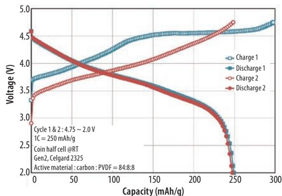
Figure 5. First and second charge–discharge profile of  $\text{Li}_{1.14}\text{Ni}_{0.29}\text{Mn}_{0.57}\text{O}_2$ .
