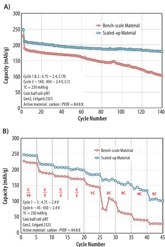
Figure 6. A) Cycling and B) rate performance comparison between the bench-scale and scaled-up materials of  $\text{Li}_{1.14}\text{Ni}_{0.29}\text{Mn}_{0.57}\text{O}_2$ .
