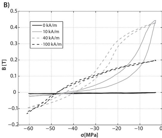
Figure 1. A) Magnetostriction of a Terfenol-d rod at different compressive stresses. B) Cyclic magnetic induction due to cyclic compressive stress (Villari effect) at different magnetic fields.
