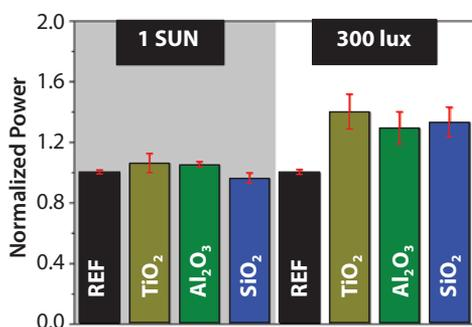
**Figure 4.** Normalized power of the DSCs using  $Al_2O_3$  (four ALD cycles),  $SiO_2$  (six ALD cycles), and  $TiO_2$  (100 ALD cycles) blocking layers deposited by plasma-assisted ALD as compared to a reference cell (REF) without a blocking layer at different irradiations (1 SUN and indoor - 300 lux with CFL lamp).
