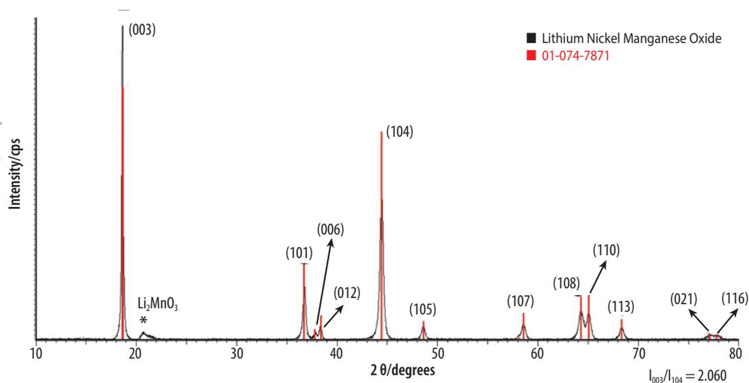
Figure 4. X-ray diffraction pattern of  $\text{Li}_{1.14}\text{Ni}_{0.29}\text{Mn}_{0.57}\text{O}_2$ .
