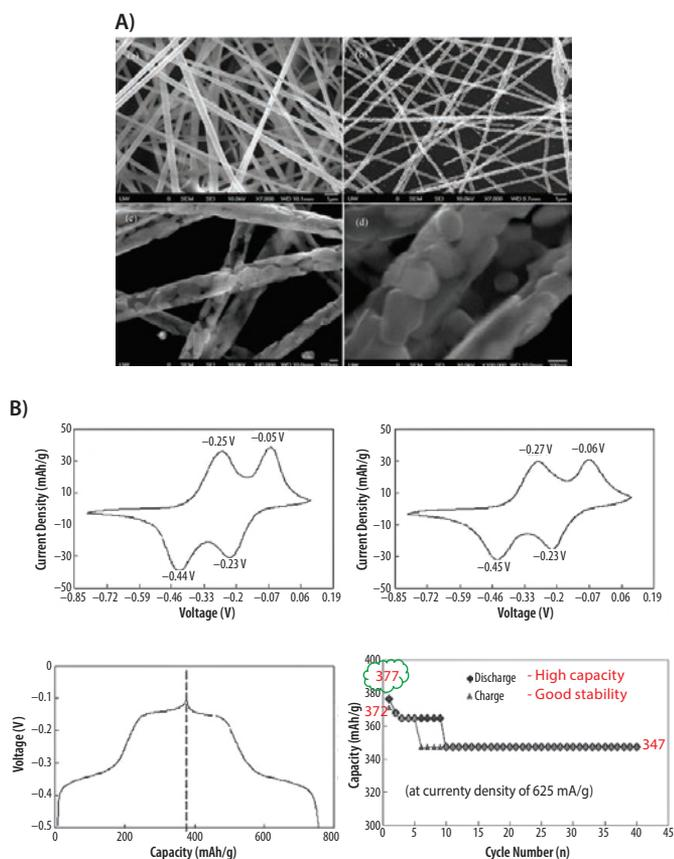
**Figure 6.** V<sub>2</sub>O<sub>5</sub> nanofibers prepared with an electrospinning method for lithium-ion battery. **A)** SEM images of V<sub>2</sub>O<sub>5</sub> nanofibers before and after being annealed (at 500 °C for 1 hr in air). **B)** Cyclic voltammetry curves and charge/discharge properties of the V<sub>2</sub>O<sub>5</sub> nanofibers at a current density of 625 mA/g.<sup>12</sup>
