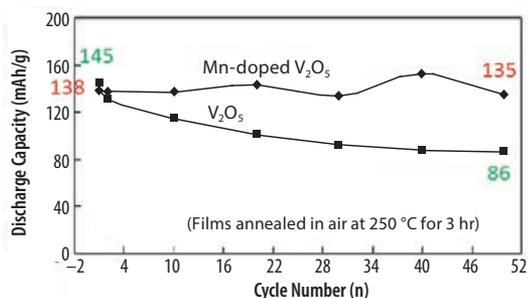
Figure 5. Enhanced cyclic stability of Mn-doped V<sub>2</sub>O<sub>5</sub> film.<sup>11</sup>
