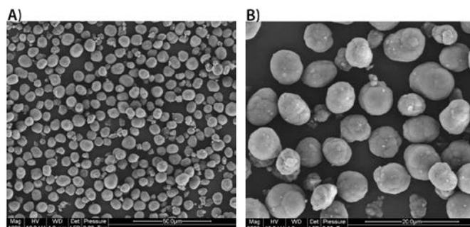
Figure 2. SEM microscopy of the dried  $\text{Ni}_{0.33}\text{Mn}_{0.67}\text{CO}_3$  precursor collected during steady-state co-precipitation (25–30 hr).
