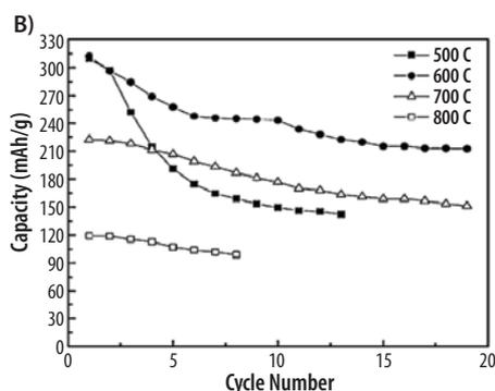
**Figure 8.**  $\text{LiFePO}_4/\text{C}$  nanocomposite for lithium ion battery. **A)** SEM images and XRD patterns and **B)** cyclic discharge capacities of  $\text{LiFePO}_4/\text{C}$  nanocomposite films annealed at different temperatures.<sup>16</sup>
