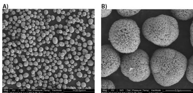
Figure 3. SEM images of the scaled-up  $\text{Li}_{1.14}\text{Ni}_{0.29}\text{Mn}_{0.57}\text{O}_2$ .
