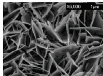
**Figure 1.** Morphology and structure of MnO<sub>2</sub> nanowall arrays produced from cathodic electrodeposition.<sup>2</sup>
