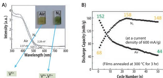
Figure 4. A comparison of the lithium-ion battery performance between V<sub>2</sub>O<sub>5</sub> films annealed in air and in N<sub>2</sub>: A) optical absorption spectra and B) lithium-ion cyclic properties of V<sub>2</sub>O<sub>5</sub> films annealed in air and N<sub>2</sub>.<sup>10</sup>
