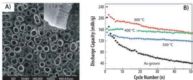
**Figure 2.** A) SEM image of a TiO<sub>2</sub> nanotube array and B) the dependence of discharge capacity and cyclic stability on annealing temperature of the TiO<sub>2</sub> nanotube array.<sup>6</sup>
