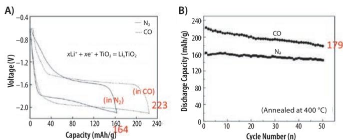
**Figure 3.** Enhanced LIB performance of TiO<sub>2</sub> nanotube arrays annealed in CO. A) The first cycle charge/discharge properties and B) cyclic stability of TiO<sub>2</sub> nanotube arrays annealed in N<sub>2</sub> and CO.<sup>7</sup>
