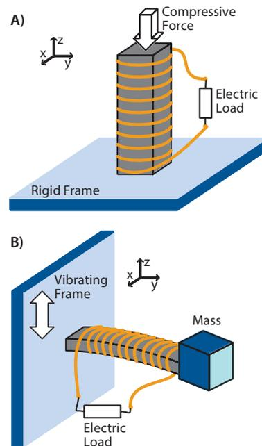
Figure 4. Two schemes for kinetic energy harvesting with magnetostrictive materials: A) force-driven and B) velocity-driven.
