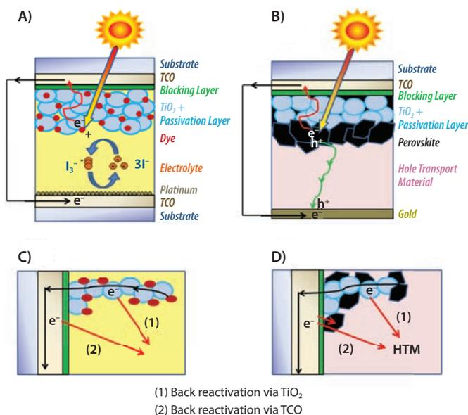
**Figure 2.** Configuration of hybrid mesoscopic solar cells: A) dye-sensitized and B) perovskite solar cells. The application of passivation and blocking layers has the purpose of limiting the primary interfacial back reactions in C) dye-sensitized and D) perovskite solar cells.
