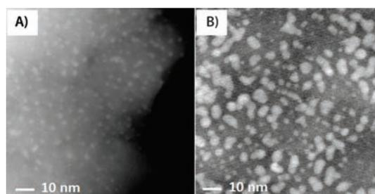
**Figure 6.** High-resolution TEM images of the platinum NPs prepared with 50 and 100 ALD cycles at 100 °C on ITO/PEN substrates.
