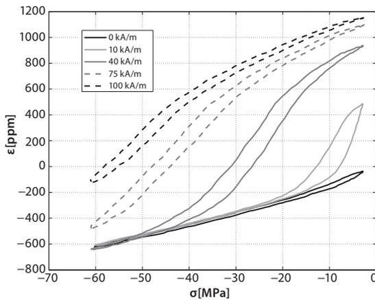
Figure 2. Mechanical characteristic of a Terfenol-d rod at different constant magnetic fields.
