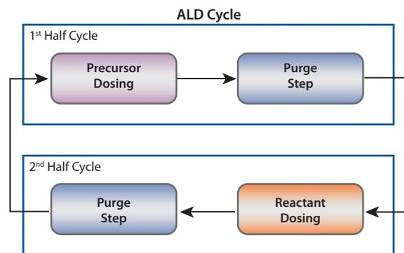
Figure 1. Schematic representation of an ALD cycle.
