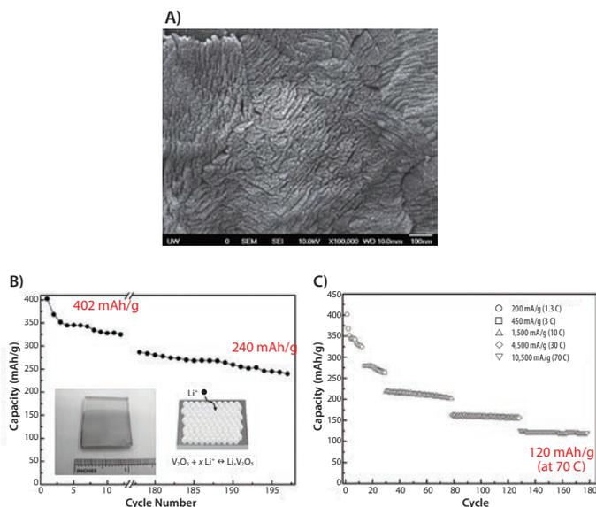
**Figure 7.** Nanoporous V<sub>2</sub>O<sub>5</sub> film for lithium-ion battery application: **A)** SEM image of nanoporous V<sub>2</sub>O<sub>5</sub> film; **B)** cyclic capacities at a current density of 200 mA/g (1.3 C); and **C)** cyclic capacities at different current densities up to 10.5 A/g (70 C).<sup>15</sup>
