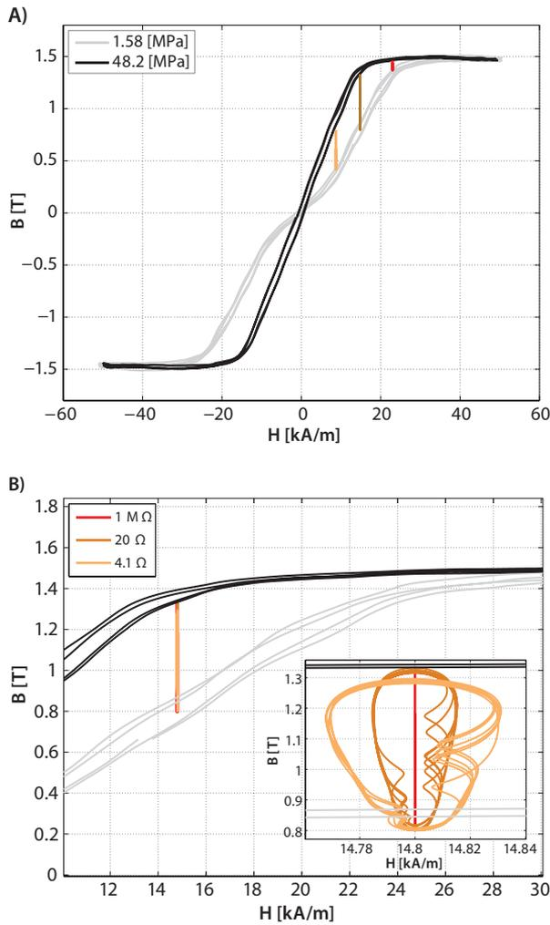
**Figure 6.** A) Magnetic characteristics of a Gallfenol rod at 1.58 MPa (black line) and 48.2 MPa (gray line) constant stresses; harvesting cycles lines:  $T = 1.25$  s,  $H = 8.7$  kA/m—orange,  $H = 14.8$  kA/m—brown and  $H = 23$  kA/m—red,  $R = 1$  MΩ. B) Harvesting cycle lines:  $T = 1.25$  s,  $R = 4.1$  Ω—orange,  $R = 20$  Ω—brown and  $R = 1$  MΩ—red.
