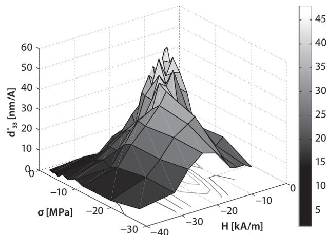
**Figure 5.** The piezo-magnetic coefficient of a Terfenol-d rod. Adapted from Reference 17.
