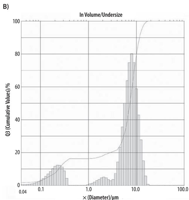
Figure 1. A) Unsteady-state precursor growth (0–25 hr) and steady-state production (25–30 hr). B) Particle size analysis of precursor slurry at 30 hr co-precipitation.
