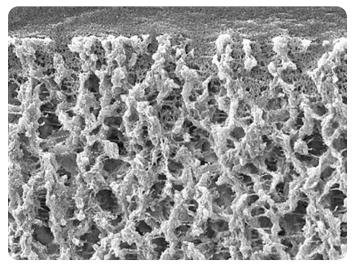
$\mathsf{Ultracel}^{\circledast}$  composite regenerated cellulose with void-free structure.
