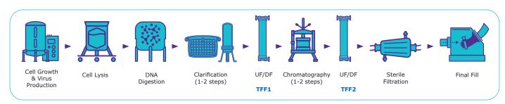
Figure 1. Typical adeno-associated virus (AAV) manufacturing process flow.
