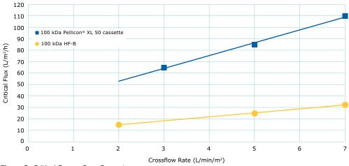
Figure 2. Critical flux vs Crossflow rate.
