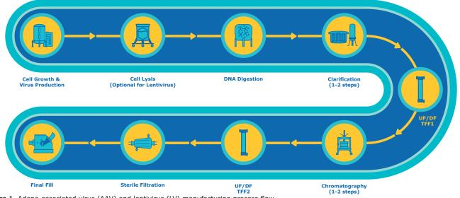
Figure 1. Adeno-associated virus (AAV) and lentivirus (LV) manufacturing process flow.
