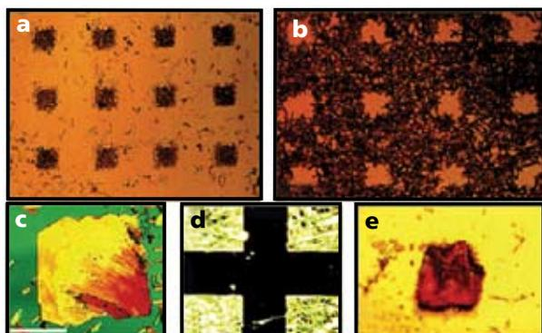
**Figure 5.** Optical micrographics of patterned arrays of organic semiconductor crystals nucleated selectively on to self-assembled terphenyl thiol template patterns: (a) and (b) anthracene crystals, scale bar = 200 μm; (c) large oriented single crystal of anthracene, scale bar = 50 μm (d) patterned anthracene crystalline films, scale bar = 300 μm; (e) patterned single crystal of 5-chlorotetracene, scale bar = 100 μm
