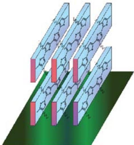
**Figure 4.** Regioregular poly(3-hexylthiophene) spontaneously assemble into ordered structures upon solution deposition. The pi-pi stacking between polymer chains facilitates charge transport.
