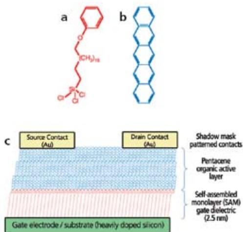
**Figure 1.** Schematic structure of an organic thin film transistor. (a) Chemical structure of the silane molecule used as the self-assembled monolayer dielectric layer (b) Chemical structure of pentacene used as the semiconductor layer (c) schematic structure of the device. Reproduced with permission from the Nature Publishing Group.
