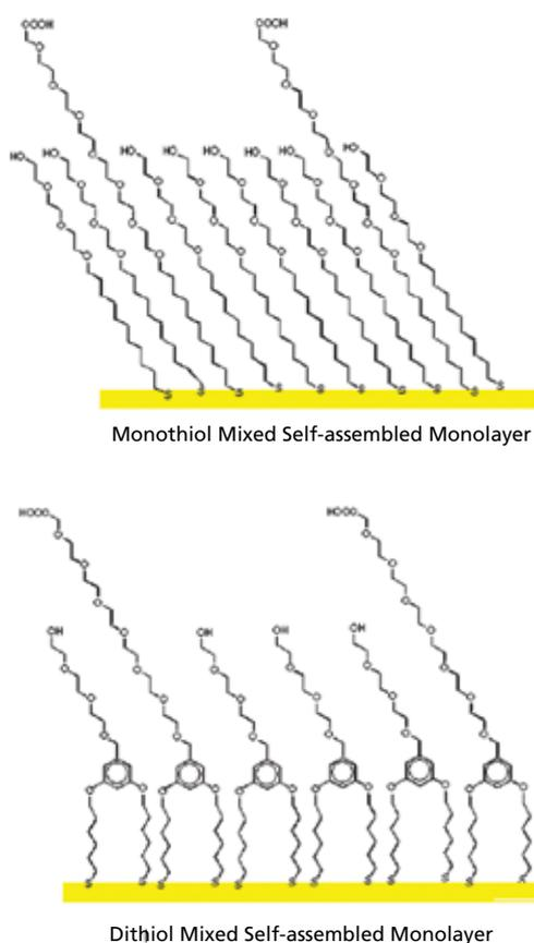
**Figure 2.** Monothiol and dithiol mixed self-assembled monolayers with PEGolated spacers.
