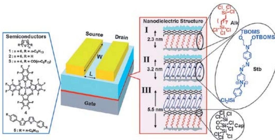
**Figure 2.** Schematic representation of the components of an OTFT showing the molecular structures of various organic semiconductors (left) and self-assembled nanodielectrics I-III (right). Nanodielectric layers were deposited from solutions of silane precursors.
