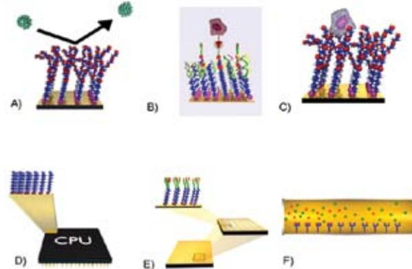
**Figure 2. Possible applications for alkanethiol monolayers.** A) Non-fouling surfaces B) SAMs with specific binding receptors C) Cell supports for native cell growth and studies D) Molecular electronics E) Microarrays F) Separations.
