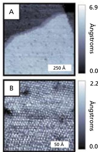
**Figure 1.** Scanning tunneling microscopy image of a 24 h 1-adamantanethiolate (1-AD) SAM on a Au{111} substrate. Image parameters:  $V_{\text{sample}} = -0.75$  V,  $I_{\text{tunnel}} = 3.0$  pA. A) Resolution:  $750 \text{ \AA} \times 750 \text{ \AA}$ ; shows several monatomic step edges and substrate vacancy islands. B) Resolution:  $200 \text{ \AA} \times 200 \text{ \AA}$ ; molecular resolution shows the 1-AD lattice.
