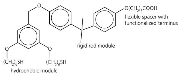
**Figure 3.** A typical rigid-rod dithiol tether (Nanotether™ BPA-HA Aldrich Prod. No. **674354**).
