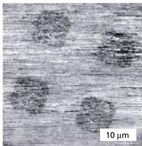
**Figure 3:** Lateral force microscopy (LFM) image of a patterned Au{111} substrate made by microdisplacement printing. The low-friction (shown as dark) squares are the stamped octanethiol molecules, and the high-friction (shown as light) background is the preformed 1-adamantanethiolate SAM. Image parameters: 40  $\mu\text{m}$  × 40  $\mu\text{m}$ , Scan rate = 1.0 Hz, Force setpoint = 4 nN.
