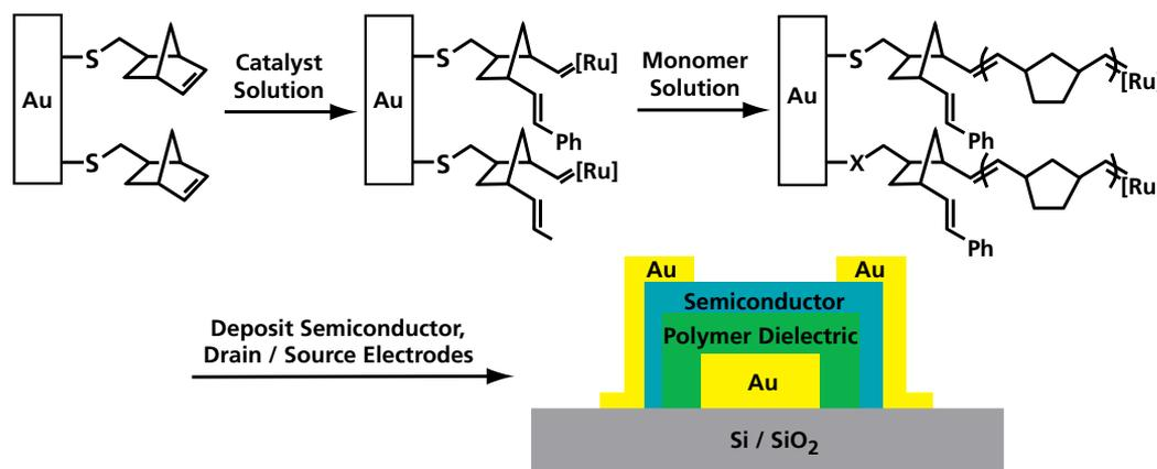
**Figure 3.** Modification of a gold gate electrode for the surface initiated polymerization reaction to grow a dielectric layer.
