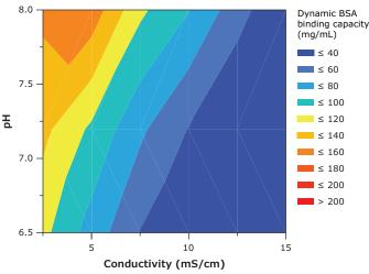
**Figure 4**: Effect of pH and NaCl concentration on BSA binding capacity (10% breakthrough) in 20mM phosphate buffer. Residence time: 6 secondes. Feed: 2 g/L BSA in 20 mM phosphate + NaCl buffer at various pH.
