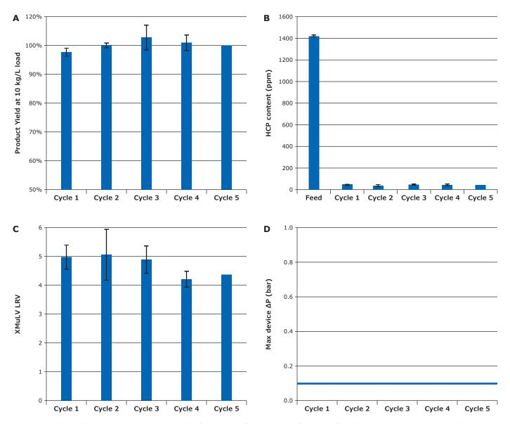
Figure 8: Product yield, HCP, XMuLV, and pressure data for a product flowthrough purification performed with a Natrix® Q Recon Mini device reused for 5 consecutive processing cycles. Mass loading was 10 kg mAb/mL membrane in each cycle. Error bars represent standard deviation of replicate tests.
