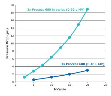
Figure 10: Pressure drop for single and serial Natrix  $^{\odot}$  Q Process 600 devices at various flowrates. Mobile phase: 25 mM Tris + 50 mM NaCl, pH 8.1.
