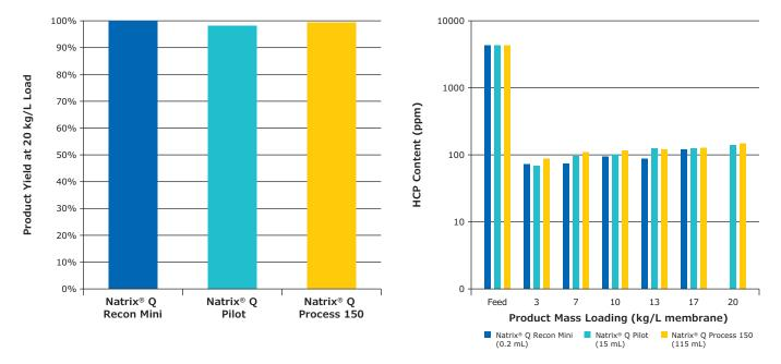
Figure 9: Yield and HCP clearance data for a mAb flowthrough purification conducted on three different Natrix® Q device scales.
