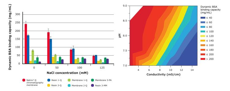
**Figure 1**: Effect of NaCl concentration on BSA binding capacity (10% breakthrough). Membrane adsorbers were operated at 6-second residence time, and resins were operated at 1-minute residence time. Feed: 1 g/L BSA in 25 mM Tris + NaCl buffer, pH 8.0.
