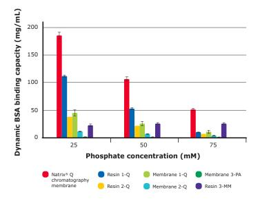
**Figure 3**: Effect of phosphate concentration on BSA binding capacity (10% breakthrough). Membrane adsorbers were operated at a 6-second residence time, and resins were operated at a 1-minute residence time. Feed: 1 g/L BSA in phosphate buffer, pH 8.0.
