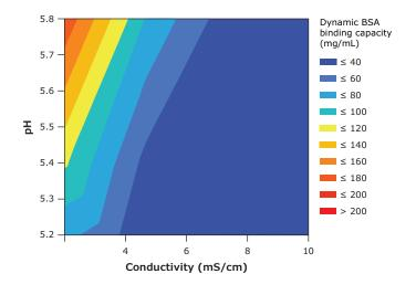
**Figure 5**: Effect of pH and NaCl concentration on BSA binding capacity (10% breakthrough) in 25mM acetate buffer. Residence time: 6 seconds. Feed: 2 g/L BSA in 20 mM acetate + NaCl buffer at various pH.
