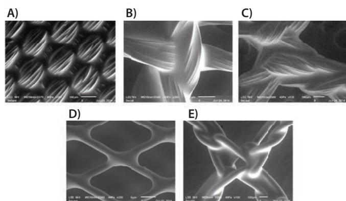
**Figure 4.** SEM images of Regenerex coatings deposited on a range of commonly used medical device textile components: **A)** dip-coated poly(ethylene terephthalate) woven, **B)** dip-coated poly(glycolic acid) knit, **C)** dip-coated PEEK mesh, **D)** spray-coated nitinol braid, and **E)** dip-coated poly(propylene) mesh. SEM images provided by Carissa Smoot of the Secant Group.
