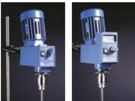
Two speed ranges for stirring applications up to 20L (in terms of H<sub>2</sub>O) of material. 292 H x 88 W x 188mm D. Wt = 2.9kg. Order stirring shafts separately; see listings in the Aldrich Handbook. CE compliant.
