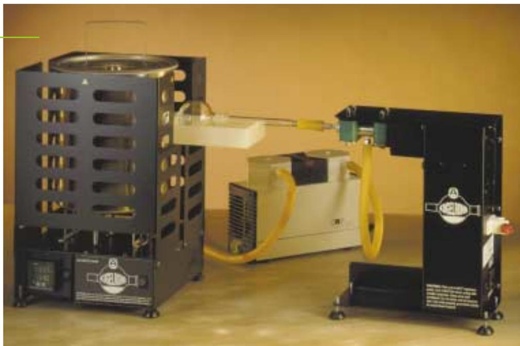
Kugelrohr apparatus shown with KNF Laboport vacuum pump (see page 4).
