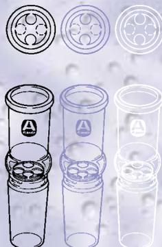
Unique design has two baffles with horizontally opposing holes that effectively prevent upward movement of foaming or bumping liquids in rotary evaporator traps. May also be used with other distillation techniques.
