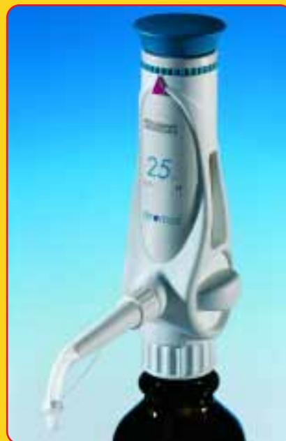
CERAMUS® bottle-top dispensers have a unique ceramic piston in a borosilicate glass barrel which guarantees the highest degree of chemical resistance, without abrasion or swelling due to solvent effects. Dispensers fit bottles with A 45 threads and include threaded adapters A 32, A 38, and S 40.
