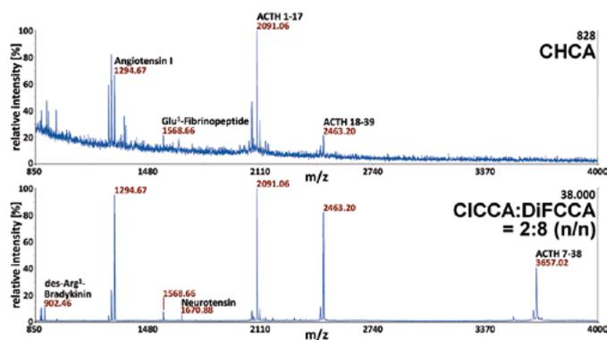
**Figure 4.** MALDI Mass Spectra of AB Sciex Peptide Mass Standard Calibration Mixtures I and II (0.5  $\mu$ l, Prepared as Given in the AB Sciex Protocol and Further Diluted by a Factor of 8) Using CHCA or CICCA:DiFCCA = 2:8 (n/n) as Matrix. Shots per Spectrum, 500; Matrix, 10 nmol Each; Mass Spectrometer, Voyager-DE STR;  $\lambda$  = 337 nm; Polarity, Negative
