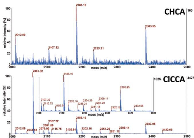
**Figure 3.** MALDI Mass Spectra of a tryptic in-solution digest of  $\beta$ -casein (Containing 10%  $\alpha$ -casein) Using CHCA or CICA as Matrix.  $m/z$  Section 2,000–2,500 Da; Shots per Spectrum, 500; Polarity, Positive; Total Sample Load, 50 fmol. For More Information, See Reference 2
