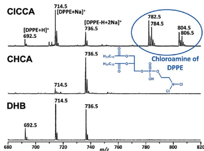
**Figure 5.** Positive-ion Mode MALDI-TOF Mass Spectra of Dipalmitoylphosphatidylethanolamine (DPPE) and Its Dichlorinated Counterpart Recorded with CICCA, CHCA, and 2,5-dihydroxybenzoic Acid (DHB). For Details, See Reference 6
