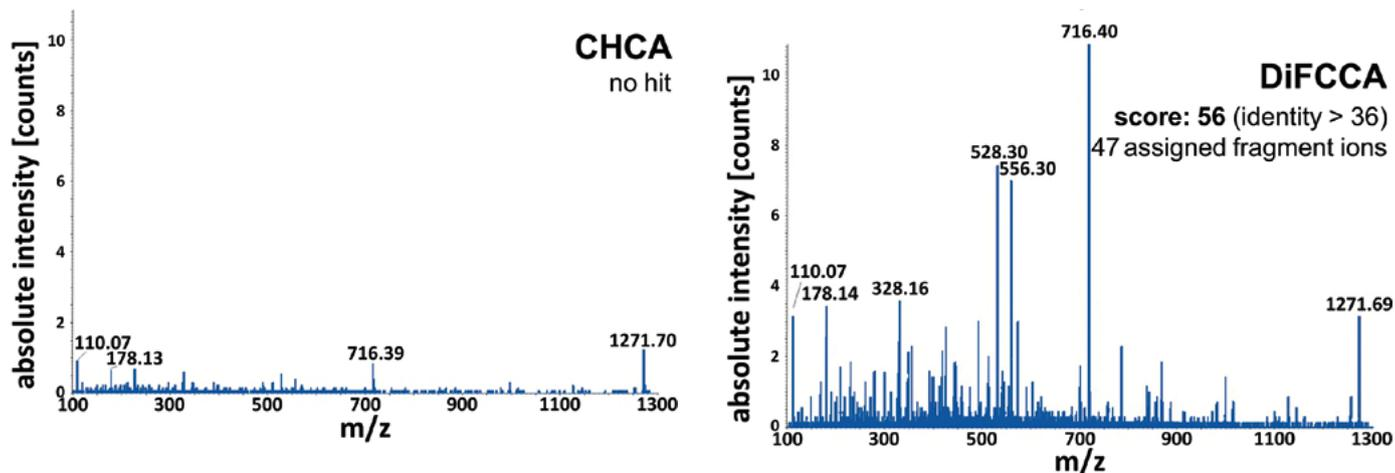
**Figure 6.** CID-MS/MS Spectra of Protonated Peptide LFTGHPETLEK ( $m/z$  1271.66) Resulting from a Myoglobin Digest (50 fmol). Mass Spectrometer, QStar Pulsar I (MALDI-QqQ-OTOF); Collision Gas, Argon; Collision Energy, 90 eV; Data base, NCBInr; Organism, Other Mammals; Enzyme, Trypsine; Max. No. of Missed Cleavages, 1; Variable Mod., CAM-C and Met.-Ox.; Precursor Tolerance, 25 ppm; MS/MS Tolerance,  $\pm 0.1$  Da
