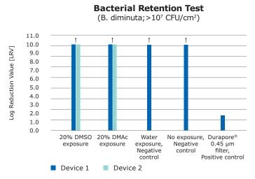
**Figure 4:** Bacterial Retention Testing Results for Opticap<sup>®</sup> XL150 Capsules with Millipore Express<sup>®</sup> SHC Membrane with and without exposure to Solvents (upward facing arrow indicates complete Retention)
