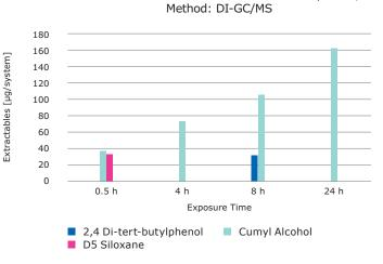
Figure 9: Extractables for Smart Flexware® Assemblies for Mobius® systems, exposed to Water
