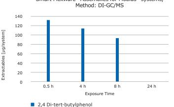
Figure 11: Extractables for Smart Flexware® Assemblies for Mobius® systems exposed to 20% DMSO
