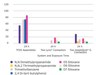
Figure 14: Extractables for Smart Flexware  $^{\otimes}$  assemblies and connectors for Mobius  $^{\otimes}$  systems, exposed to 20% DMAc
