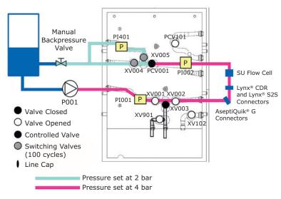
Figure 8: Valve Cycling Test Setup
