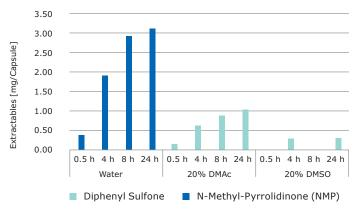
Millipore Express<sup>®</sup> SHC Membrane Non-Volatile Extractables via HPLC-DAD/MS
