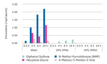
Figure 2: Semi-volatile extractables for Opticap® XL5 Capsules with Millipore Express® SHC membrane
