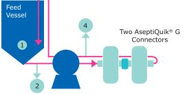
Figure 6: Schematic of Lynx $^{\circledast}$  and AseptiQuik $^{\circledast}\,G$  Connectors Setup used during solvent recirculation
