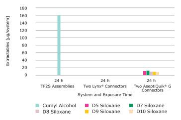
Figure 10: Extractables for Smart Flexware® Assemblies and Connectors for Mobius® systems, exposed to Water
