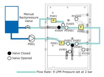
Figure 7b: Valve Bypass Testing, Configuration 2
