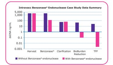
Figure 8. Case study data summary showing effective reduction of DNA by  ${\tt Benzonase}^{\circledast}$  endonuclease.
