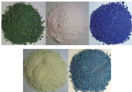
**Figure 4.** Photographs of 3DOM zirconia, silica (top middle) and titania powders (bottom left). The different colors of the 3DOM zirconia samples arise from the different pore sizes.
