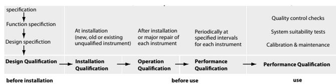
**Figure 4.** Timeline of Analytical Instrumentation Qualification (AIQ)
