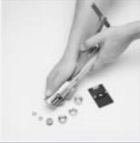
For occasional production of KBr pellets. Prepares KBr discs of 1, 3, and 7mm diameter, depending on die set used. Requires only a firm, steady hand pressure on the handle. Complete with 1, 3, and 7mm die set and pellet holder.
