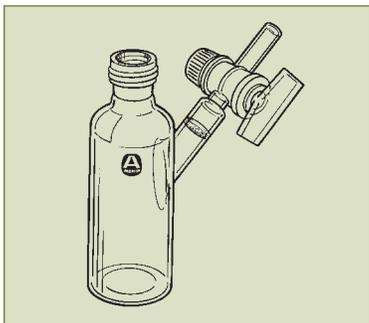
The "Schlaker" tube (derived from "Schlenk" and peptide "shaker") is designed for running oxygen-sensitive reactions on a solid-phase resin. The glass frit in the sidearm permits filtration of excess reagents and solvent removal with complete recovery of the resin for the next reaction. Made of heavy-wall glass, with glass stopcock and frit (porosity 25 to 50  $\mu\text{m}$ ) on sidearm, and a plain or threaded  $\frac{1}{4}$ "/20 top joint. Compatible with Schlenk glassware.
