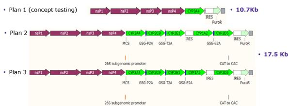
Simplicon Design: Two larger RNA constructs were created, each containing five CYP450 enzymes (Plan 2 and Plan 3) separated by either a 2A peptide cleavage site, or an IRES sequence. Additionally, a smaller construct containing only the CYP3A4 enzyme was designed to begin experiments while the larger constructs were being assembled. A puromycin resistance gene was included on all constructs.
