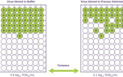
• quench analysis evaluates how the effects of an inactivating substance present in the process intermediate can be mitigated.
