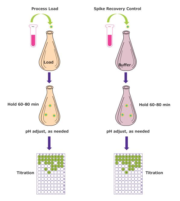
Figure 5. An example of a spike recovery assay for process loads (not including virus reduction filtration or a membrane chromatography). Virus is spiked into process load material and buffer at the same ratio used in the clearance study and then held in a biosafety cabinet before being assayed for infectious virus.
