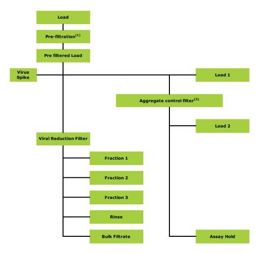
**Figure 10**. Schematic of the Experimental Design for the Evaluation of Viral Clearance by a Viral Reduction Filter. 1) The pre-filtration is the process-specific pre-filter used to "protect" the viral reduction filter. 2) The aggregate control filter is not part of the manufacturing process and is a size exclusion filter carefully selected to remove any viral aggregation that may have formed on addition of the virus to the sample
