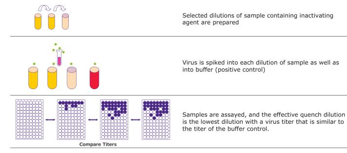
Figure 7. Schematic of quench analysis assay.
