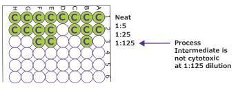
Figure 2. Overview of cytotoxicity assay. In this example, the process intermediate is not toxic at a dilution of 1:125. This will be the starting dilution for the viral interference assay.
