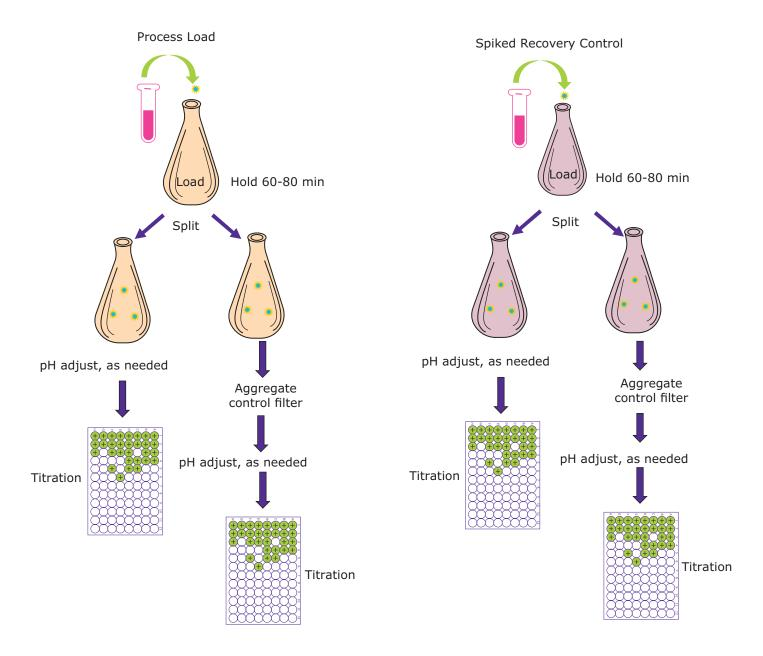
Figure 6. An example of a spike recovery assay for a virus reduction filtration or a membrane chromatography load. Virus is spiked into process load material and buffer at the same ratio used in the clearance study and then held in a biosafety cabinet before being assayed for infectious virus.
