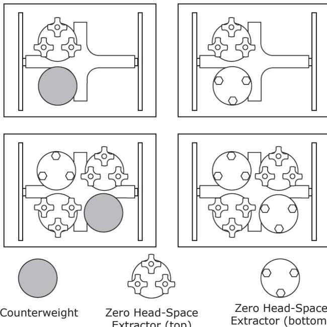
3. Align the top plate of one ZHE unit with the bottom plate of the adjacent unit. The edges of the top and bottom plates of the ZHE units should lie next to the strips of padding in the chambers. The top and bottom of each ZHE unit should be flush with the edges of the spindle.
