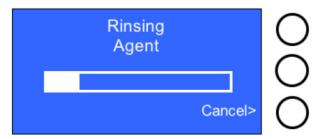
The rinsing agent rinses Nebulizer 1 first, and then Nebulizer 2. There is a pause while the pad holder remains under Nebulizer 2 to ensure thorough rinsing before continuing. The rinsing agent is collected by the absorbent pads.
