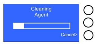
The cleaning agent flows first through Nebulizer 1, and then through Nebulizer 2. There is a pause while the pad holder remains under Nebulizer 2 to allow sufficient contact time for thorough cleaning before spraying resumes. The cleaning agent is soaked up by the absorbent pads.
