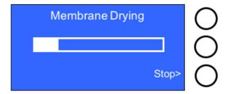
The membrane spins and goes to Position 2 where it moves in a short arc back and forth under a stream of filtered air that dries the membrane until the end of the preprogrammed time.
