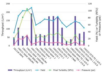
Figure 5. Throughput vs. yield, final pool turbidity and final pressure of tested filtration options
