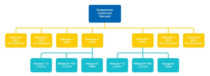
Figure 2. Structured design of the clarification experiment
