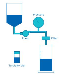
Figure 1. Pmax<sup>™</sup> experimental set-up
