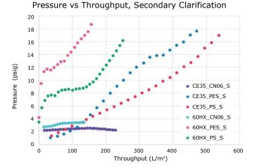
Figure 4. Pressure vs. throughput of secondary clarification options, following primary clarification
