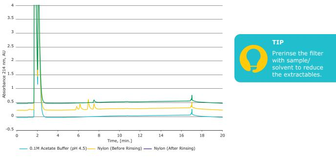
**Figure 4**. **Nylon syringe filters are a common source of extractables.** In this experiment, the extractable peaks seen after filtration through nylon were greatly reduced when the first milliliter of filtrate was discarded and the second milliliter was analyzed.
