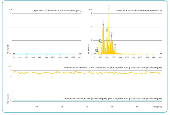
Figure 13. Comparison of MS spectra (top) and TIC chromatograms (bottom) of the two buffer systems,
