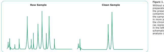
Without sample preparation, the presence of contaminants in the sample results in more peaks in the chromatogram (as represented in the left hand schematic), making analysis challenging.
