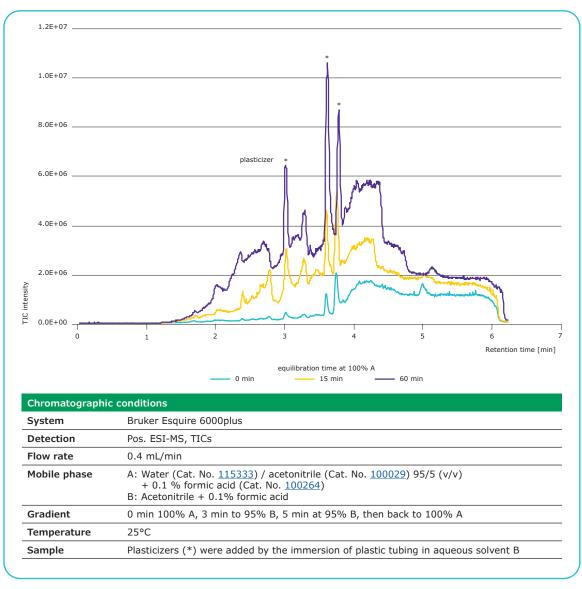
Figure 14. Accumulation of contaminants on an HPLC column for various periods of time and elution via a gradient profile.
