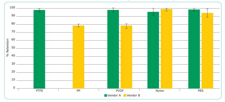
**Figure 2.** Particle retention ability differs between different membranes and between different suppliers. In principle, 100% of filtration membranes should retain particles. To test this hypothesis, microporous membranes from two different vendors (pore size 0.2 µm) were tested for latex particle retention following filtration of a suspension of 0.3 µm latex particles in water. PTFE=polytetrafluoroethylene; PP=polypropylene; PVDF=polyvinylidenefluoride; PES=polyethylenesulfone.
