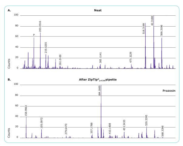
**Figure 9.** ZipTip<sup>®</sup> pipette tips increase sensitivity of mass spectrometric analysis. Plasma sample from rat dosed with 10 mg/ kg prazosin was injected into an LTQ/Orbitrap mass spectrometer by nanoelectrospray (a) before and (b) after preparation using a C18 ZipTip<sup>®</sup> pipette tip. Adapted from Erve JCL et al, Rapid Commun. Mass Spectrom. 2008; 22: 3015–3026.
