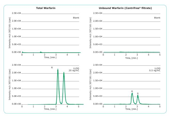
**Figure 5.** LC-MS analysis of total vs. free warfarin present in blank matrix (top) and human plasma samples (bottom). Unbound (free) warfarin was separated from protein-bound warfarin using centrifugal ultrafiltration devices, such as the Centrifree<sup>®</sup> device. Adapted from Jensen BP, Chin PK, Begg EJ. Quantification of total and free concentrations of R- and S-warfarin in human plasma by ultrafiltration and LC-MS/MS. Anal Bioanal Chem. 2011 Oct;401(7):2187-93.
