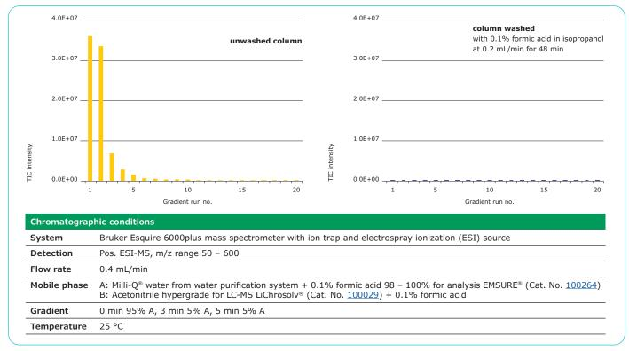
**Figure 16.** Column washing can compensate for column bleeding. Total ion current (TIC) of a competitor column after 20 gradient runs: left- unwashed column; right- column washed with 0.1% formic acid in isopropanol at 0.2 mL/min for 48 min.
