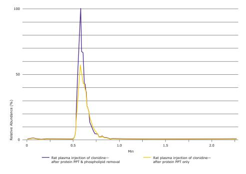
**Figure 10.** Removing phospholipids can improve the signal-to-noise ratio in LC-MS.
