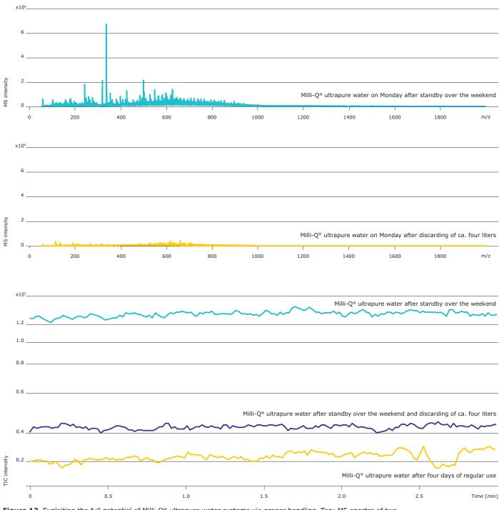
**Figure 12.** Exploiting the full potential of Milli-Q<sup>®</sup> ultrapure water systems via proper handling. Top: MS spectra of two samples of ultrapure water delivered at different points of time; bottom: TICs of the same samples and one additional sample. All analyses were performed via direct injection of the preconcentrated solvents into the MS operated in positive ESI mode.
