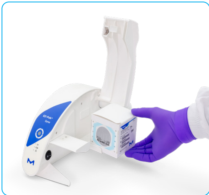
Step 1 Open cover and insert the cartridge.
